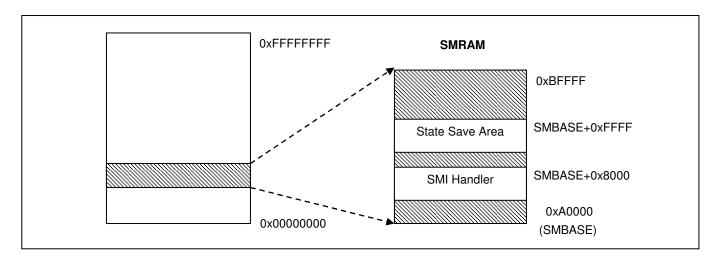
Figure 1: The physical memory map for the Intel 845 chipset showing location of the compatible SMRAM region and its layout on a 32-bit system.
