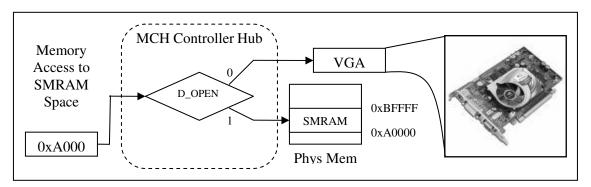
Figure 2: SMRAM memory accesses are filtered by the chipset based on their origin and the state of D\_OPEN in the SMRAMC register. SMM accesses are normally directed to SMRAM while non-SMM accesses are directed to VGA memory.
