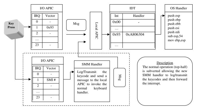
Figure 3: Normal and SMBR keystroke handling paths
