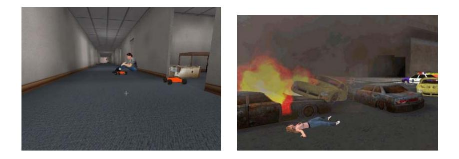
Simulated version of the competition using Unreal Tournament game environment Simulated robot, sensors, control API and environment are given Competitors design control code and user interface http://sourceforge.net/projects/usarsim
