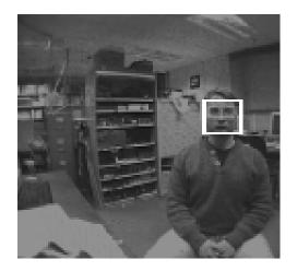
Figure 6: An example face in a cluttered environment. The 128x128 grayscale image was captured by the active vision system, and then processed by the pre-filtering and ratio template detection routines. One face was found within the image, and is shown outlined.
