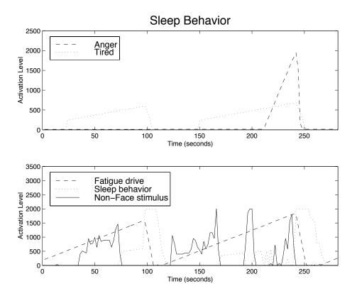
Figure 18: Experimental results for long-term interactions of the fatigue drive and the sleep behavior. The fatigue drive continues to increase until it reaches an activation level that potentiates the sleep behavior. If there is no other stimulation, this will allow the robot to activate the sleep behavior.
