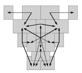
Figure 5: A 14 pixel by 16 pixel ratio template for face detection. The template is composed of 16 regions (the gray boxes) and 23 relations (shown by arrows). Essential relations are shown as solid arrows while confirming relations are shown as dashed arrows. Adapted from Sinha (1996).
