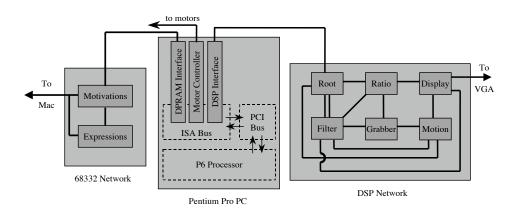
Figure 3: Computational hardware utilized by Kismet. A network of digital signal processors acts as the sensory processing engine and implements the perception system, the attention system, and part of the motor system. This network is attached to two 68332-based microcontrollers that implement the motivational, behavioral, and remainder of the motor systems.
