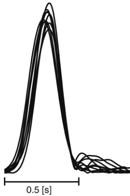
Fig. 12. Trial by trial hand velocity profiles of subject: each line indicates the hand velocity profile of the reaching movements for the target pair 'b', generated by subject A. The velocity profiles are aligned at the time when the tangential velocities decrease and become 0.15 m/s during the later half of the movements.
