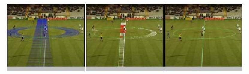
Figure 5: Estimating the camera parameters by taking the current parameters, projecting the field model using the current parameters onto the image (left), finding the correspondences between model points and the imagepoints (middle), and adjusting the camera parameters to achieve minimal errors (right).
