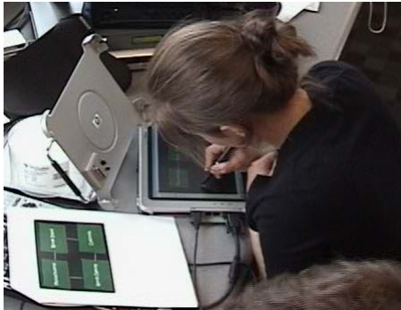
Figure 1: The physical setup. Shown here is a pen technique and the subject has chosen to lay the Tablet PC on the table surface. (Out of view are the standard-sized keyboard and mouse used for non-pen techniques.)
