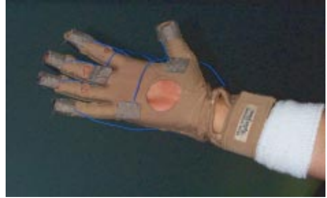
Figure 1: The Flex and Pinch input system. Although a CyberGlove[4] is shown, any bend-sensing glove can be used.
