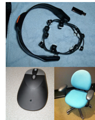
figure 2. Several devices were used to elicit physiological data. We instrumented a mouse (left) with a heat/humidity sensor and a chair with pressure sensors (right). The Emotiv EPOC (top) was also used.
