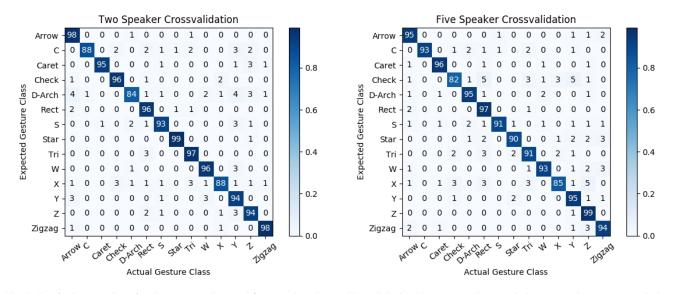
Table 4: Confusion matrices for the two speaker and five speaker data collected during the user study. Y-axis is expected gesture, x-axis is actual recognized gesture. Results are user dependent. There is very little structured confusion between gestures. C, Double Arch, and X have the most confusion in our two speaker setup. Check and X have the lowest accuracy in the five speaker configuration.
