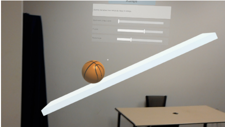
Figure 1: AR image capture of the headset presenting a ramp with a bouncing ball which interacts with the spatial mesh captured by the HoloLens.
