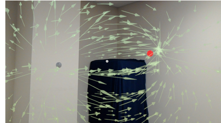
Figure 2: AR image capture of the headset presenting a point charge electrical field as an illustration of Coulomb's Law.
