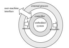
Figure 1. Main components of an embedded system
