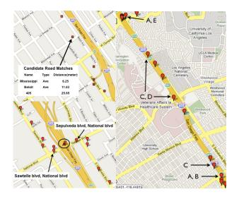
Figure 3: Example of naive map-maptching failure (top-left), intersection-based map-matching (bottom-left), and intersection with nearest road and substitution (right)
