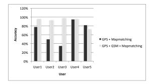
Figure 4: GPS-based versus GPS and GSM-based accuracy
