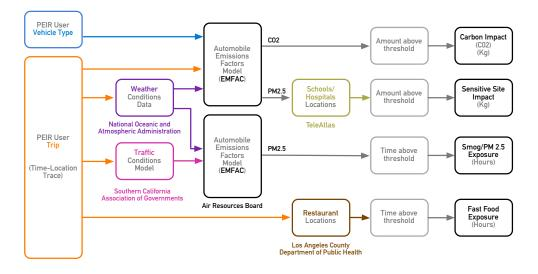
Figure 6: Data flow diagram
