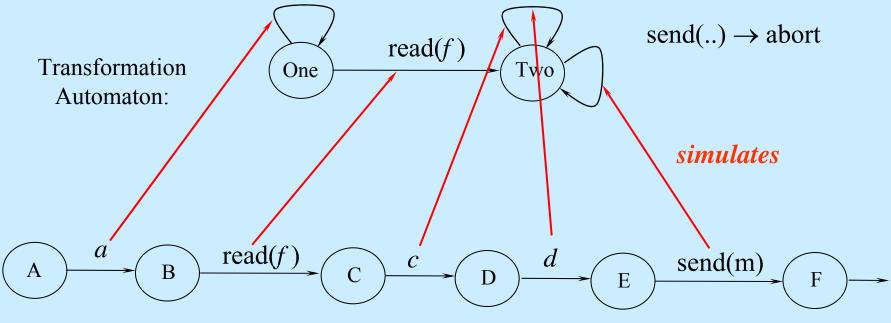
Build simulation map, then generate new code for corresponding actions send(m) action is replaced by abort action
