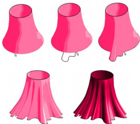
Figure 9: A skirt modeled with cross sectional oversketch. Top row, left to right : starting with a simple tube, the user selects a cross section of the surface. Next, the user redraws a section of it and this edits the surface. Bottom row : the surface is rotated and drawn upon further, and the results are shown with both toon and Gouraud shading for clarity.
