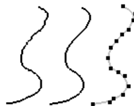
Figure 2: Stroke capture: unfiltered stroke (left), after applying the reverse Chaikin filter (middle) and the final stroke showing its control points (right).
