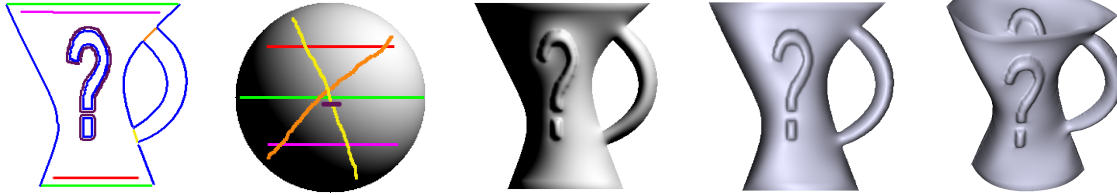
Figure 1: An example of 3D markup using Shape Palettes . The ‘question mug’ is created by linking 2D primitives drawn in the freehand view to their corresponding 3D shape on the “shape palette” (the sphere). For example, the 3D orientation of the top and bottom curves of the mug correspond to the 3D orientation of the green curve on the shape palette. Specifying this relationship will generate a cylinder-like structure. Adding only a few more strokes for extra details and the ‘question mug’ is created.
