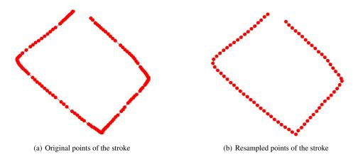
**Figure 1:** *The original points (a) are varied in distance away from each other, whereas the resampled points (b) are interspaced evently.*
