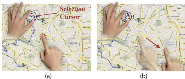
Figure 5: Interaction with FingerMap : The coarse hand specifies an area of interest. (a) The user touches the zoomed-out view with the tracking finger, and a selection cursor appears in the center of the area of interest. (b) FingerMap applies any translation of the fine hand to the cursor on a smaller scale. Once the cursor overlaps with the desired waypoint, the user selects it by releasing the coarse hand.
