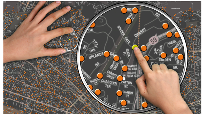
Figure 1: Interaction with FingerGlass : The user specifies an area of interest with one hand and interacts with the magnified objects with the other hand. During the interaction, a new area of interest can be defined. Releasing all fingers makes the tool vanish.
