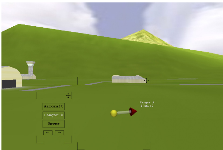
Fig. 1. The “3D arrows” navigation aid: 3D arrows are used to point towards target objects or places and associated text is used to provide information about target name and distance from the user.
