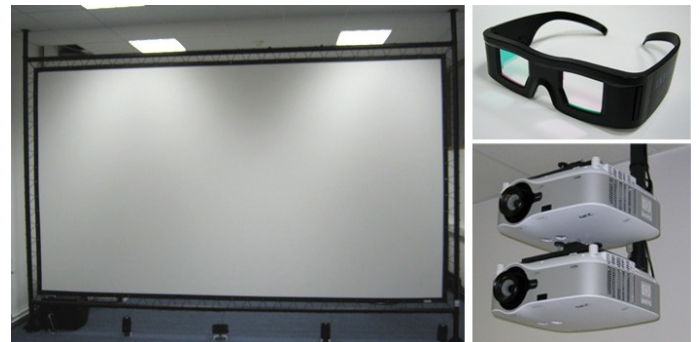
Fig. 7. Parts of stereoscopic system: screen, glasses and projectors
