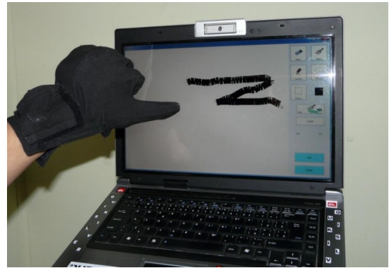
Fig. 10. Drawing with data glove using drawing system
