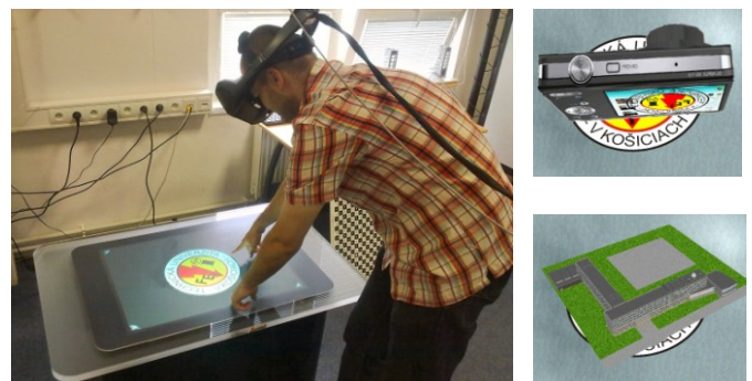
Fig. 11. Augmented reality system (left) and examples of user views (right)
