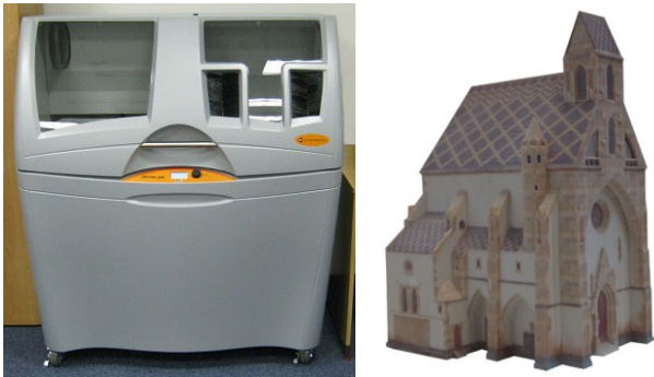
Fig. 8. ZPrinter 450 (left) and 3D model printed by this 3D printer (right)
