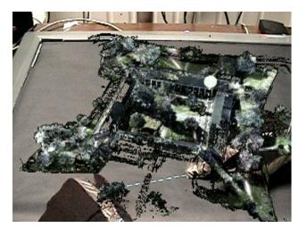
Figure 11: Balloon Selection being used in a dense point cloud model of Fort Jay at Governors Island, NY. (Range scan data courtesy of Columbia University Robotics Lab.)
