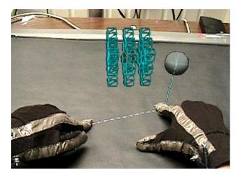
Figure 1: Balloon Selection in action. 3D spherical cursor above the surface is controlled by multi-finger interaction on the touchsensitive surface. This image is taken through a video-mixed augmented reality system on a black paper-covered projection surface.
