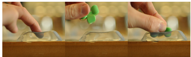
Figure 3. The thermoplastic Elastomer deforms when force is applied but returns to normal state quickly, as seen in the middle image.
