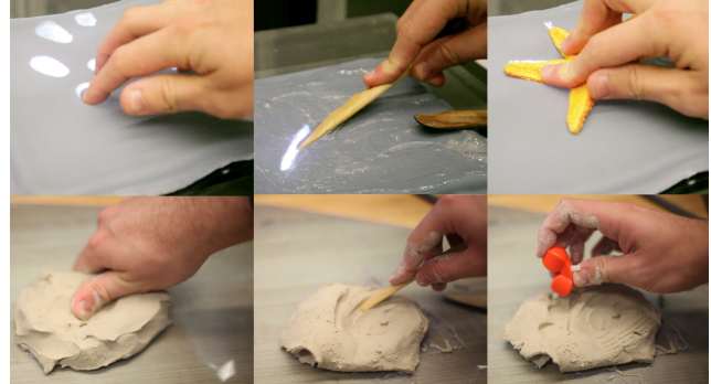
Figure 1. Above: Using hands, tools and arbitrary objects to input with deForm. Below: Using hands, tools and arbitrary objects to deform clay.
