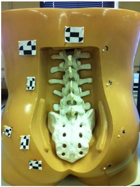
(a) Picture of the torso mannequin with a spine model in the cutout. CT beads are visible on the right and the MicronTracker markers are shown on the left.
