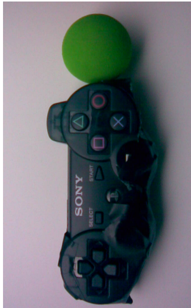
Figure 36: Very early PlayStation Move prototype, based on a "modified" SIXAXIS controller.
