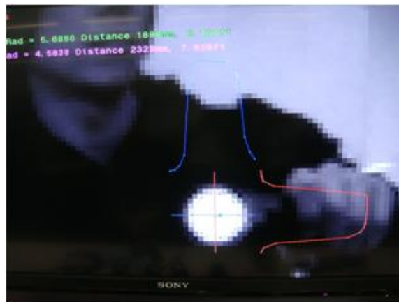
Figure 37: Visualizing the 2D pixel intensity distribution of the PlayStation Move sphere is useful for debugging the model fitting stage.
