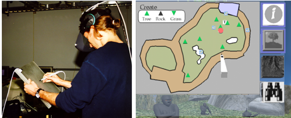
Figure 13: The Pen and Tablet Metaphor. The image on the left shows the user holding the pen and tablet and the image on the right shows what the user's sees in the virtual world.
