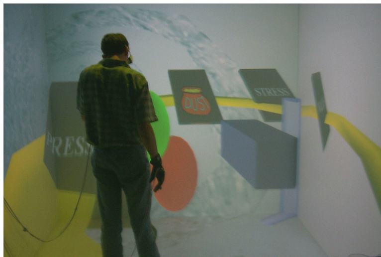
Figure 12: An example of a virtual toolbelt. The user looks down to invoke the belt and can grab tools and use them in the virtual environment.
