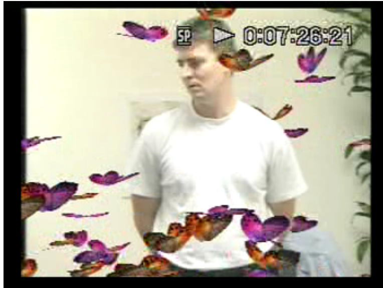
Figure 24: 3D pixel data allows real video to be mixed with virtual graphics with proper pixel occlusion. Some of the butterflies pass in front of the person, while others fly behind him.
