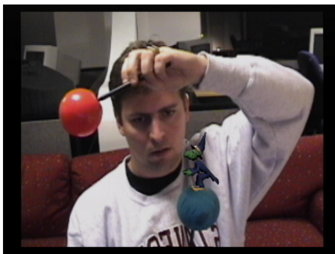
Figure 19: 3D color tracking for augmented reality. The virtual witch character "stands" on the blue sphere and "watches" the red sphere.
