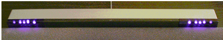
Figure 28: The Wiimote sensor bar has two groups of IR LEDs at fixed widths.
