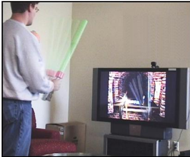
Figure 17: Color tracking using EyeToy. A virtual game sword moves in response to the green toy.
