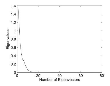
Figure 3-3: Eigenvalues Associated with the Principal Components
