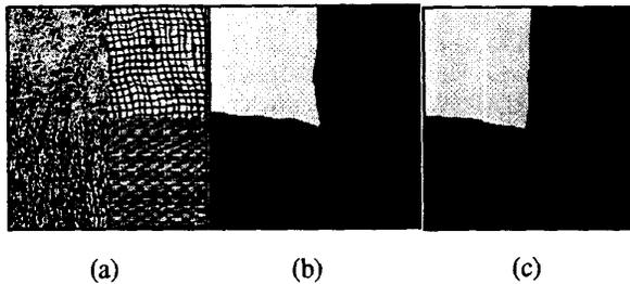
**Figure 5. Segmentation of an image consisting of 4 textures from the training Set. (a) Original image, (b) Segmented image using 1-NN, (c) Segmented image using the FAMNN - m**
