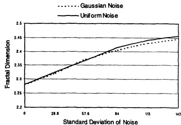
Figure 2. FD versus standard deviation of noise
