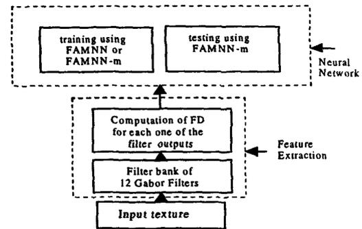
Figure 1. Block diagram of classification method
