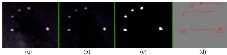
**Figure 3.** A camera frame passed through the image processing pipeline: raw camera frame (a), background filtered (b), threshold (c), processed points (d)
