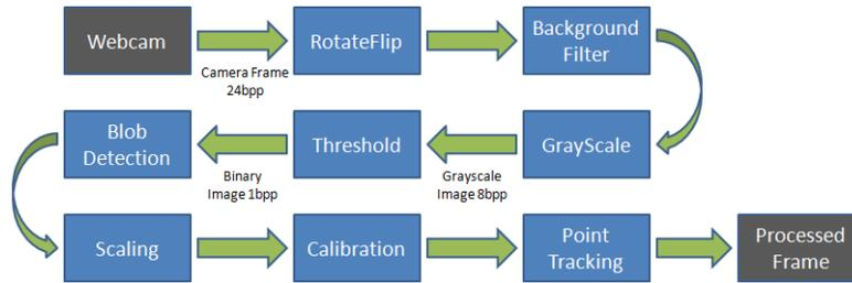
Figure 2. Image processing pipeline
