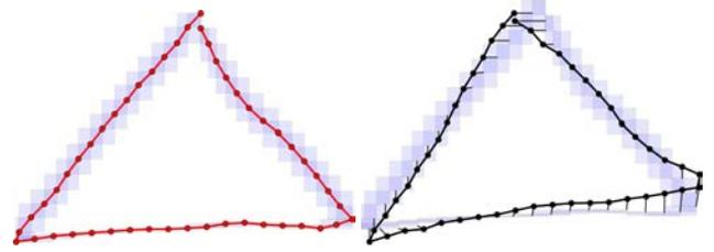
**Figure 2:** Visualization of a  $LB_{Keogh}$  lower bound in 2D for the triangle gesture from \$1-GDS [38]. On the left, the combined upper and lower bands of a template form a light blue bounding box per point. On the right, the  $LB_{Keogh}$  lower bound is calculated for a query as the sum of the minimum squared Euclidean distance from each point in  $Q$  to the corresponding point boundary from  $T$  (shown as thin black lines).
