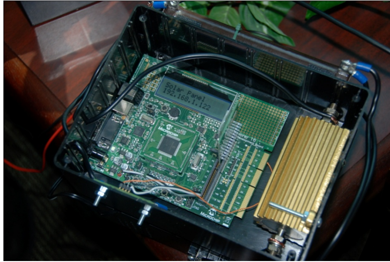
Figure 72 – Solar Panel Device Explorer 16 Board
