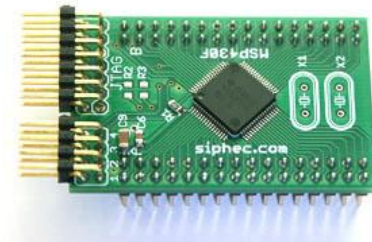
Figure 2.32: Picture of the TinyBoard with one of the MSP430 class processors. (Provided by Siphec, permission pending).
