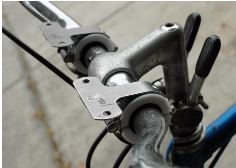
Figure 4.2: These two clamps on the bike provide a surface to attach our device to.
