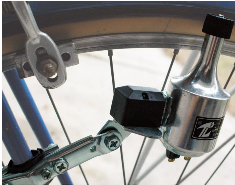
Figure 2.2: A ‘bottle generator’ attached to the rear wheel of a bicycle.
