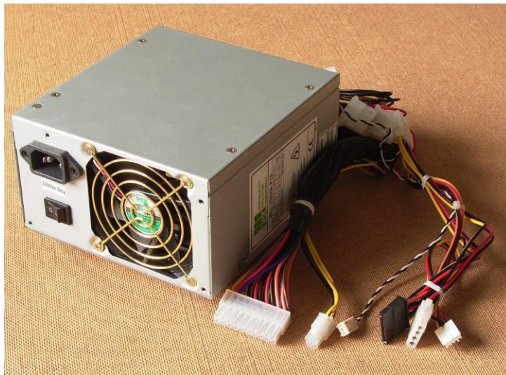
Figure 2.6: An example of a switched-mode power supply. (Image falls under the GNU Free Documentation License for distribution.)
