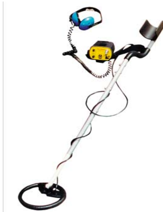
Figure 3.2.3.1 Pulse Induction Metal Detector Printed with permission
