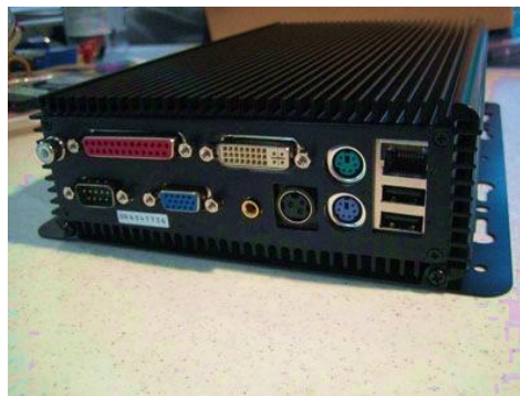
Figure 59 - Fins used to dissipate heat and keep elements out
