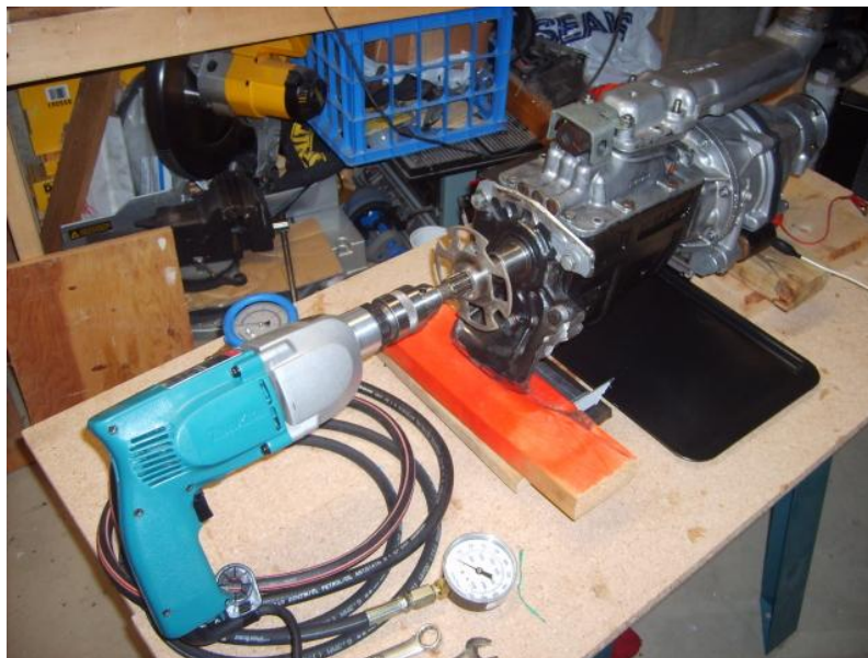
Figure 63 – RPM Testing Method
