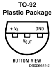
Figure 2. LM34 temperature sensor (Bottom view)
