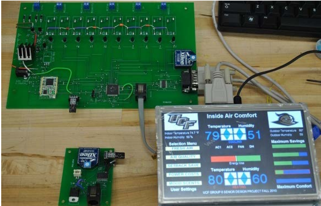
Figure 2.1: Generation 1 HVAC Control System (iTemp)
