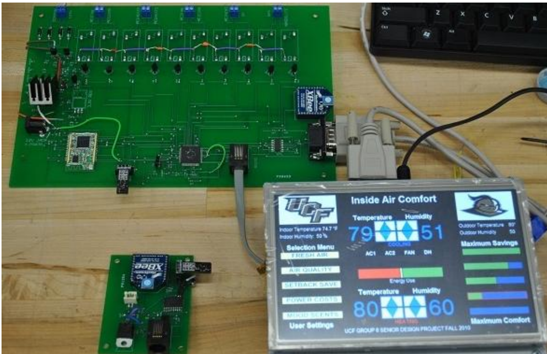
Figure 2.1: Generation 1 HVAC Control System (iTemp)
