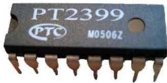
Fig. 4. PT2399 Echo Processor
