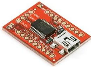
Figure 4. FT232RL USB to Serial Converter
