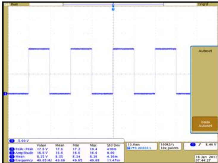
Figure 7.3.3-1 PWM waveform on oscilloscope
