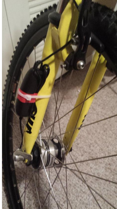
Figure 25 - Hub Dynamo and AC/DC Converter
