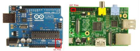
Figure 43 I2C Embedded Communication Pins
