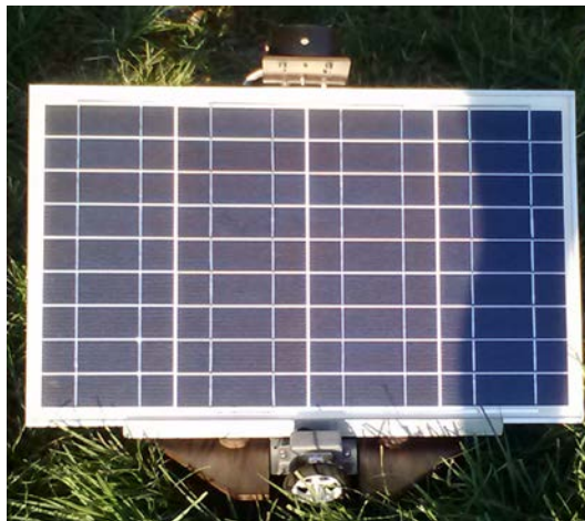
Figure 4.8.1.5-4; Final Solar Tracker Assembly
