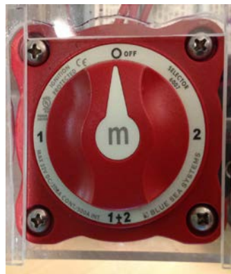
Figure 8-2; Image of the main power switch
