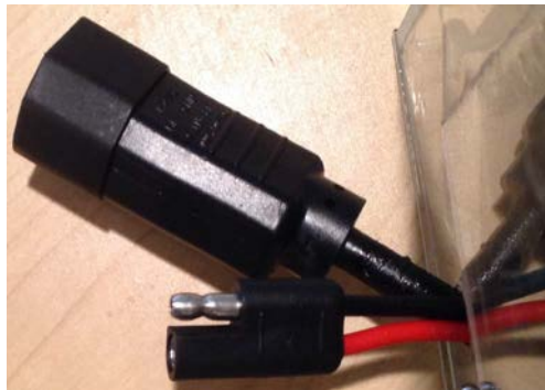
Figure 8-1; Power cord sockets; the above one is for the AC wall connection and the other forms the connection to the solar tracker
