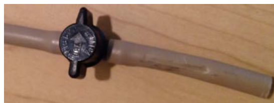
Figure 8-3; Image of the water tank release valve in the closed position
