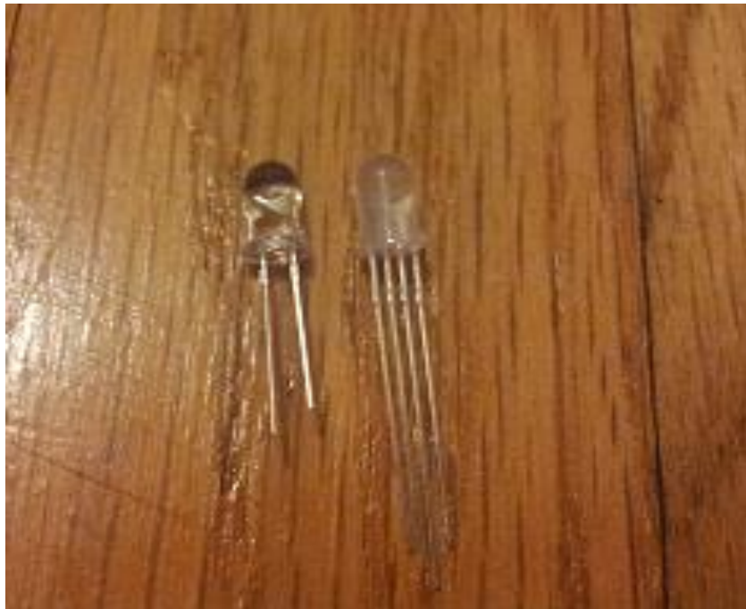
Figure 3.5: Clear (left) vs. Diffused RGB (right) Light Emitted Diodes
