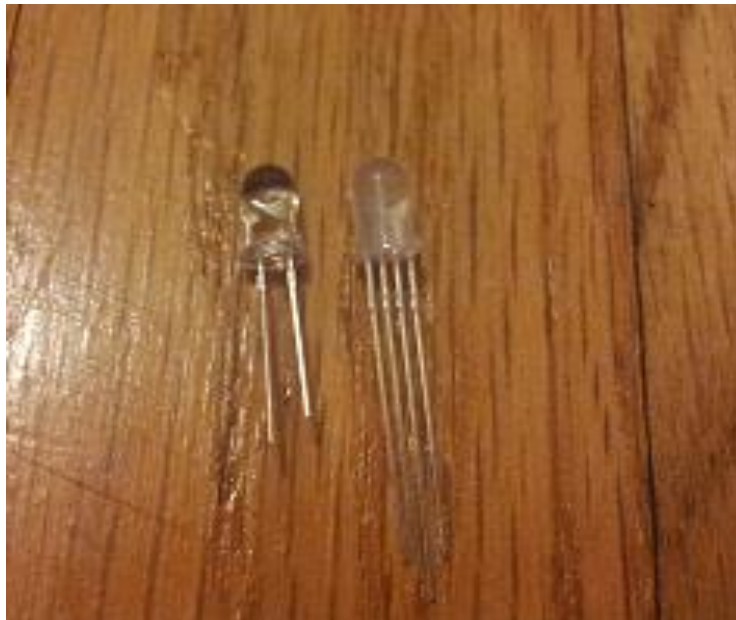
Figure 3.3: Clear (left) vs Diffused RGB (right) Light Emitted Diodes
