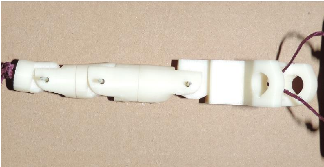
Figure 7. Assembled finger with the proper wiring for motion control.
