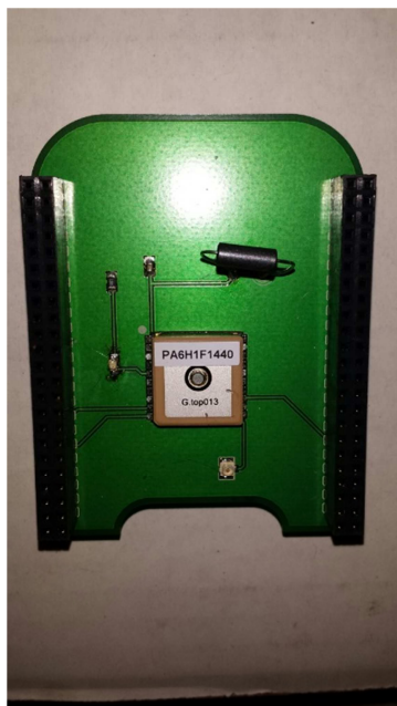
Figure 5: MTK3339 GPS Module PCB with headers
