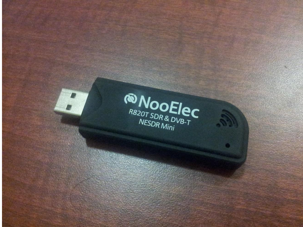
Figure 7 – Low Cost ADS-B Receiver Dongle
