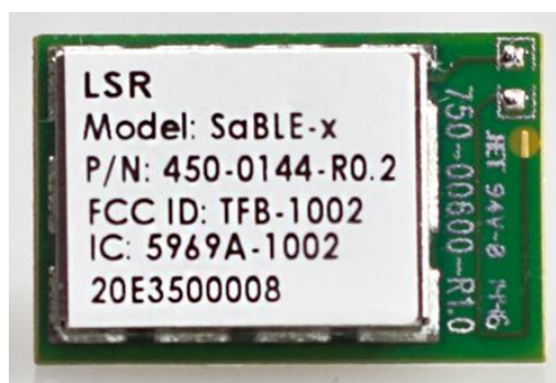
Figure 15: SaBLE-x module from LSR Reprinted with permission from LSR
