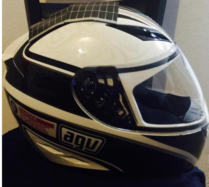
Figure 34: Solar Panel Placement Side View
