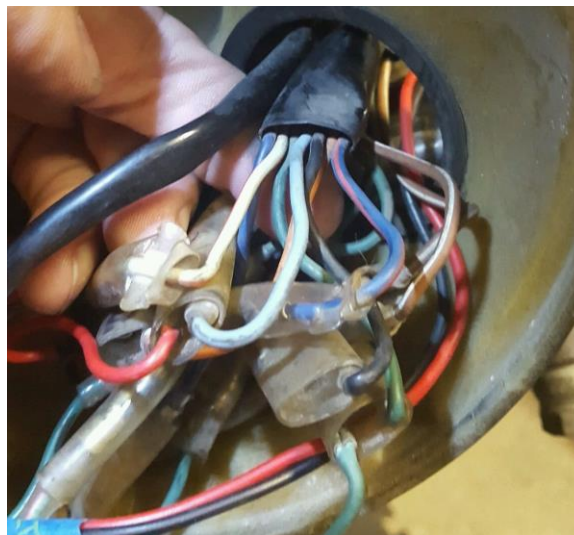
FIGURE 21: HONDA CB400F WIRES CONNECTING TO THE LEDS
