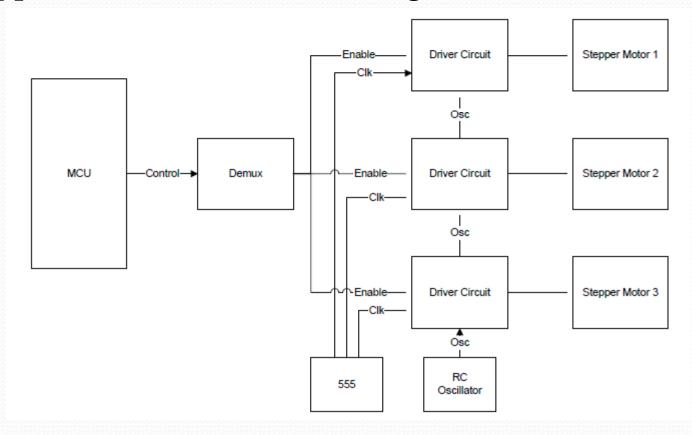
Stepper Motor Circuit Diagram
