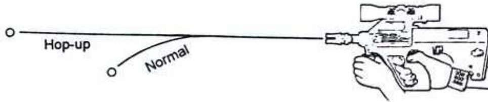
Figure 4.4.2.5: Illustration from the gun manual showing the contrast between hop-up and normal shots. Reprinted with permission from www.airsoft.com
