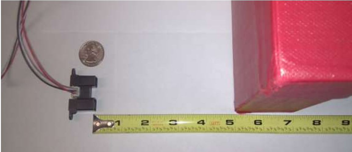
Figure 4.6.1.1: Calibrating the distance versus output voltage of the Sony GP2Y0A02YK (measuring at an invalid distance).
