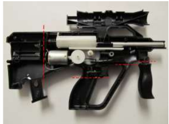
Figure 4.4.2.2: The red dashes indicate where the gun can be cut to reduce size and weight
