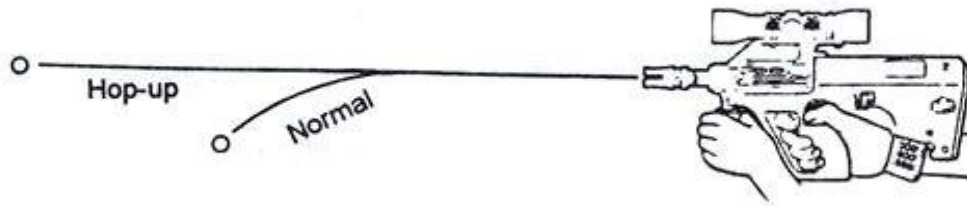
Figure 4.4.2.5: Illustration from the gun manual showing the contrast between hop-up and normal shots. Reprinted with permission from www.airsplat.com
