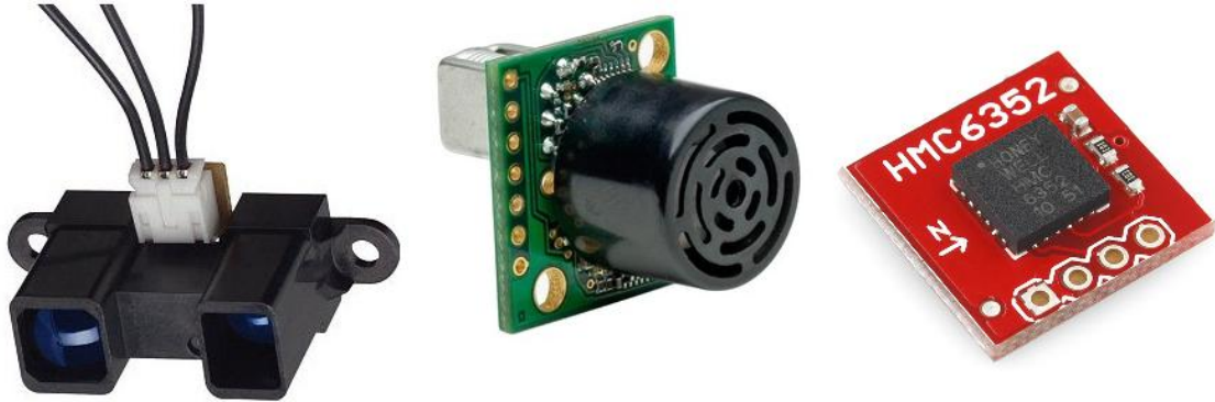
Figure 5.0.2.4: GP2Y0A02YK on left, MB1210 center, and HMC6352 on right Permission pending
